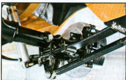
CalTracs rear suspension features adjustable preload with split monoleaf and traction bars. Note added section in middle of wheelwell.
